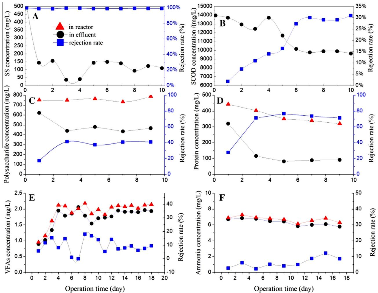
Fig. 4. Retention efficiencies of SS (A), SCOD (B), polysaccharides (C), proteins (D), VFAs (E), and ammonia (F) by the dynamic membrane.
