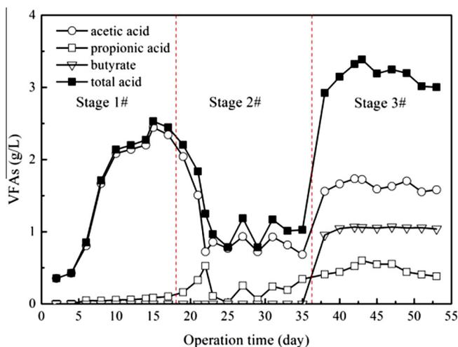
Fig. 2. Performance of the AFSFDMBR in sludge fermentation for VFA production.
