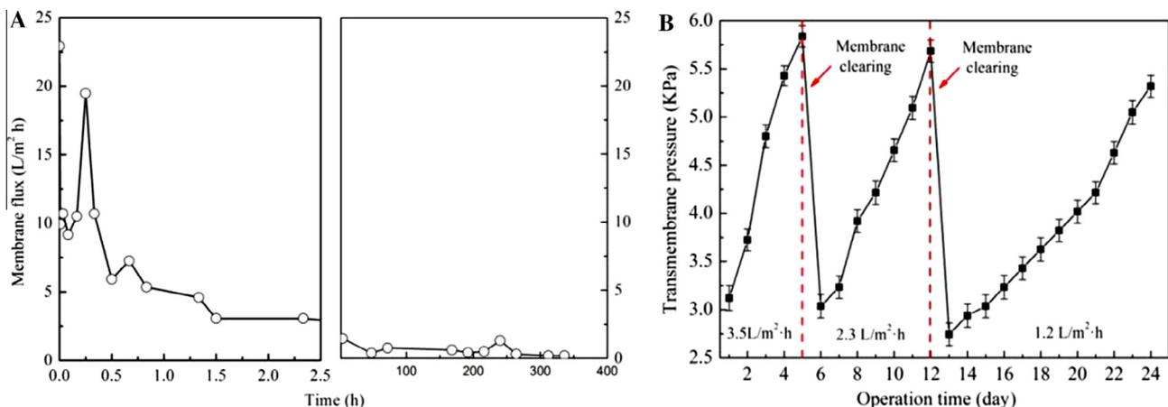
Fig. 3. Variation of the membrane flux under constant membrane resistance during one operation period (A), and variations of membrane resistance under a constant membrane flux (B).
