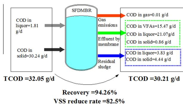
**Fig. 6.** COD balance during stage 3 in the AFSFDMBR.
